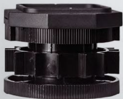
Adjusting foot – Composed of the adjusting foot pedestal and the installation fastener, which can be used for vertical installation, and an adjusting function of the height can also be realized. Adjusting foot pedestal – It is used for supporting the floor plate during installation, and height can be adjusted freely.
