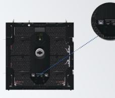
Power and signal connectors bottom location makes it quick for and easy access.
