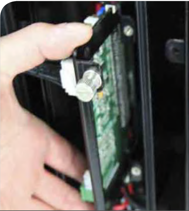
Full redundancy Hot-swappable Control & Power Supply System
