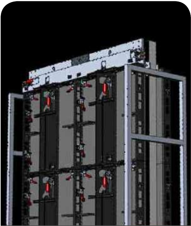
Unique Time & Space-saving Touring Transportation Rack with Dual Passive Suspension System carrying Two Pre-rigged Sections of 2-by-2 panels.
